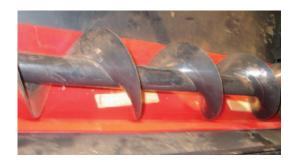
3. Insert liner (AGTCP10100) under the auger and use shims to wedge panel down tight against floor as shown in the picture to the right. Be sure the panel is inserted so the shape of the liner matches the trough.
